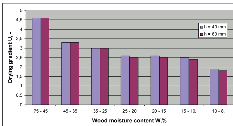
Fig. 1. Change in the drying gradient of the suggested regimes depending on wood moisture content and on the thickness of lumber
