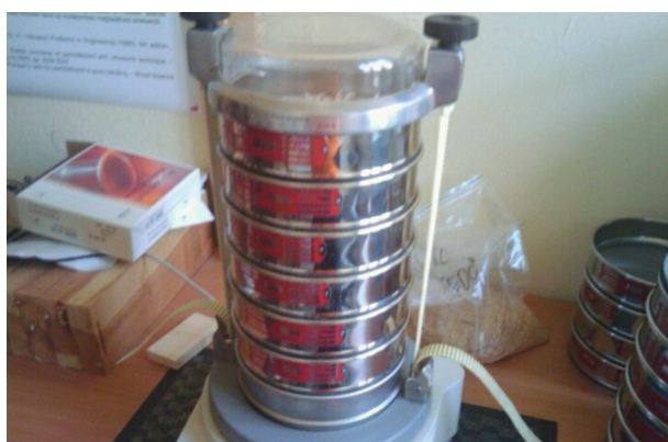
Figure 2. The Fritsch Analysette 3 PRO sieve column
